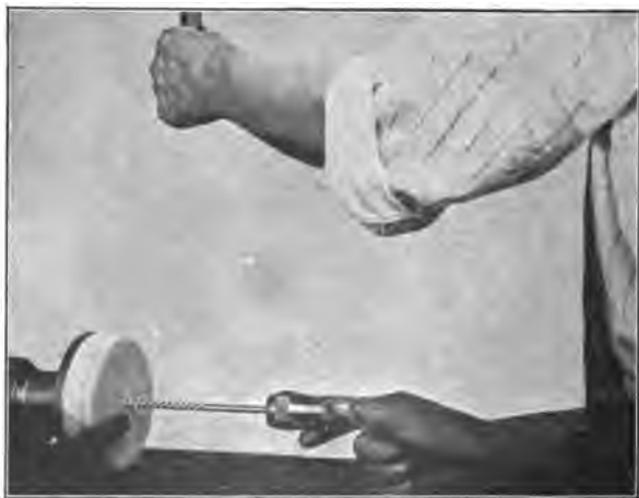
Fig. 273. Boring with Bit.
